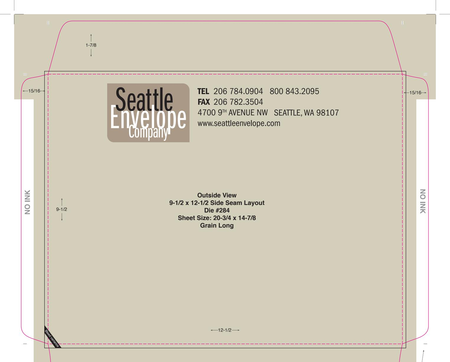
**Bleeds** - We can not guarantee perfect bleeds. Slight variation occurs naturally in the die cutting & folding process. For best results, allow 1/8" tolerance. The quality of the printed stock directly affects the process; with press bounce & missing side guidelines having a negative impact. Variance can be minimized by using our Profile Die system on larger orders (25,000 +) or sending in stock that has been letterpress die cut and scored. Grain direction is critical for Profile Dies.
